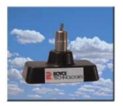
The standard ultrasonic, dual crystal sensor used with the 2501A and 2511A Interface Level Analyzers for all normal aqueous non-chemical conditions, where maximum temperatures do not exceed 175° F (80° C). It incorporates a 3/4″ 316 Stainless Steel nipple for customer supplied pipe mounting.
