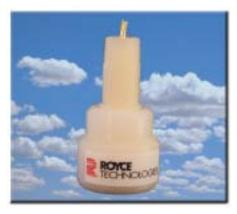
For generally harsh environment applications, this solid, Kynar sensor is made of chemically inert epoxy. It incorporates a 3/4" Kynar pipe nipple for customer supplied pipe mounting. All cables are high temperature Teflon jacketed. It can be used in chemical solutions of temperatures to 220° F (105° C).
