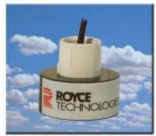
Designed specifically for the Model 2505 analyzer, this economical sensor uses a single crystal to both transmit and receive. Constructed of the same material as the 25DN; it is used in non-chemical applications where the maximum temperatures do not exceed 175° F (80° C). Its physical size allows the sensor to be inserted into a pipe with an I.D. of 3 inches. It incorporates a 3/4″ 316 Stainless Steel nipple for customer supplied pipe mounting.
