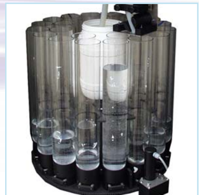
24 x 2 litre borosilicate glass bottles (DURAN 50) and optional an additional PE composite container of 6.4 litres.
